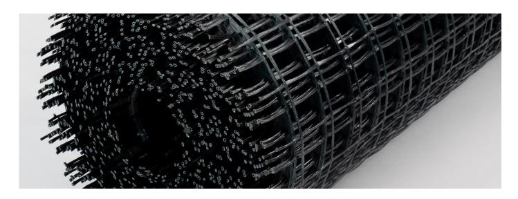
This specific mesh is intended to reinforce floor screeds, cement, and lime plasters. Big mesh sizes of 40×40 mm facilitate mesh sinking in concrete. The standard technique of strengthening screed floors with steel wire trusses is challenging to install and costly to transport. Compact size and light weight enable rapid and straightforward installation and prevent the high costs of transporting big objects.
